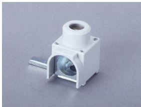
31 028 connecting terminal, side connection for comb-type busbars 31 014, 31 024, 31 309, 31 311 6 - 50 mm 2
